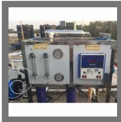
Commercial Reverse Osmosis System
